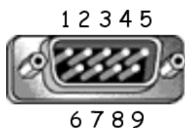
DB9 Male Connector J1 (bottom of product label, sensor side)
