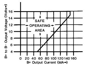
To operate safely in the "unsafe" area of the curve, at low voltage settings, use an external resistor in the B+ line, to take most of the drop externally, and connect the + sense line in the normal manner. Do not allow prolonged shorts across the output.
